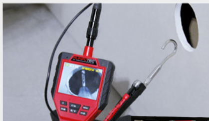
Cavity wall inspection, locating and capturing
